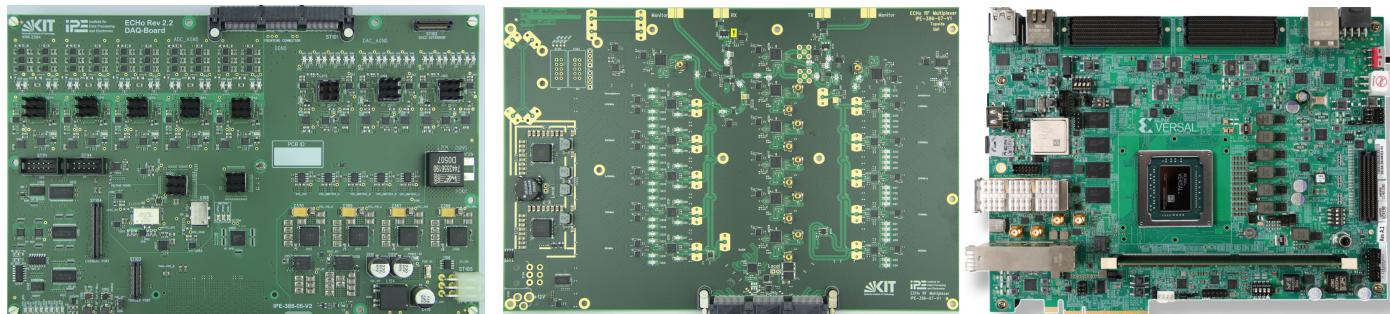
One central topic of our research is the development of room-temperature readout systems for cryogenic experiments. In particular, we focus on the control of qubits and readout of frequency multiplexed quantum sensors, which require powerful systems with custom firmware for driving the multiplexers and real-time analysis of the detector data. Current efforts are on scaling the systems for reading out 1000 of sensors respectively operating several tens of qubits simultaneously.
