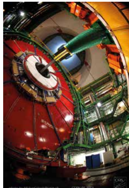
Photo of the 16-m-high CMS detector. Visible above is the access shaft through which all elements of the detector have been lowered. The collision hall is 100 m below the ground.
