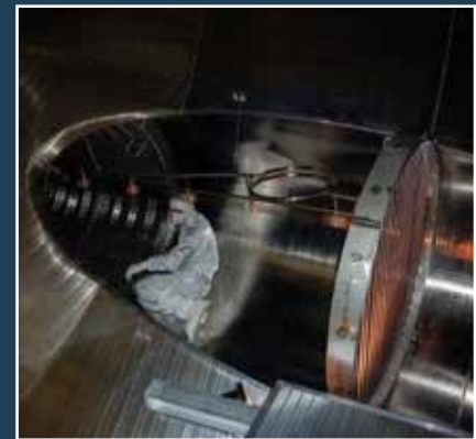
KATRIN Main Spectrometer – view at one of the pumping ports with getter pump frame (left) and a liquid-nitrogen cooled copper baffle.
