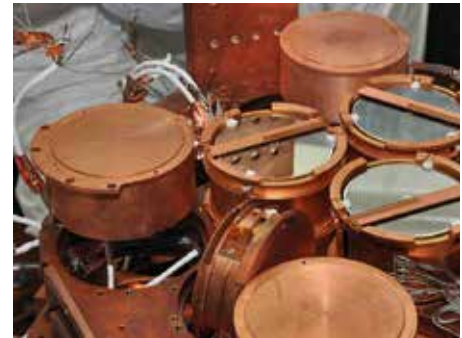
Assembly of high-purity germanium crystals for Dark Matter search with EDELWEISS
